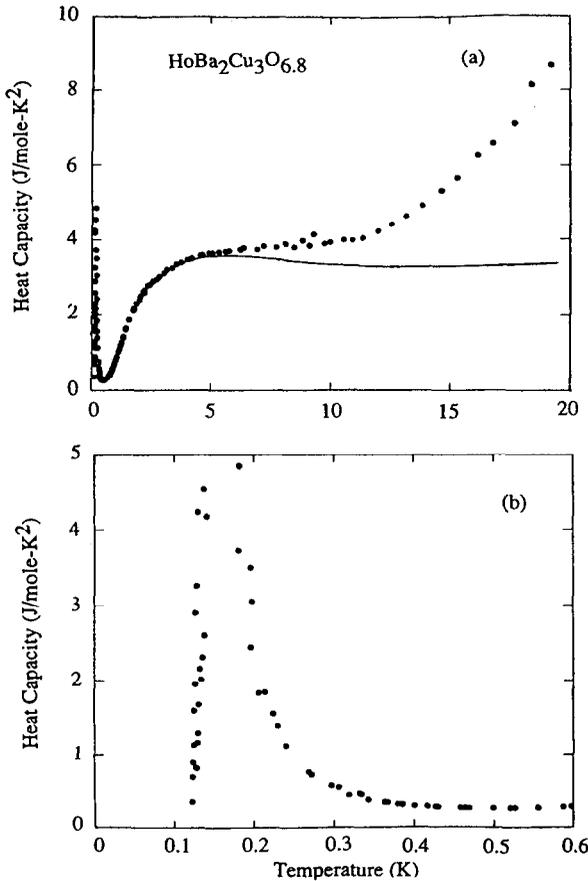
Fig. 5. Heat capacity vs. temperature for  $HoBa_2Cu_3O_{7-x}$ . The solid line shows the result of subtracting the heat capacity of  $YBa_2Cu_3O_{7-x}$ .
