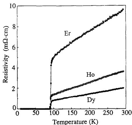
Fig. 1. Resistance vs. temperature for  $REBa_2Cu_3O_{7-x}$  compounds.
