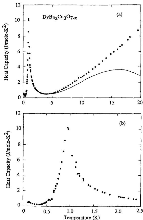
Fig. 4. Heat capacity vs. temperature for DyBa<sub>2</sub>Cu<sub>3</sub>O<sub>7-x</sub>. The solid line shows the result of subtracting the heat capacity of YBa<sub>2</sub>Cu<sub>3</sub>O<sub>7-x</sub>.
