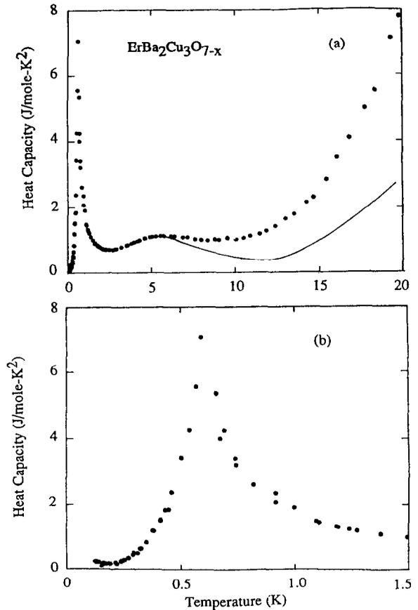
Fig. 6. Heat capacity vs. temperature for  $ErBa_2Cu_3O_{7-x}$ . The solid line shows the result of subtracting the heat capacity of  $YBa_2Cu_3O_{7-x}$ .
