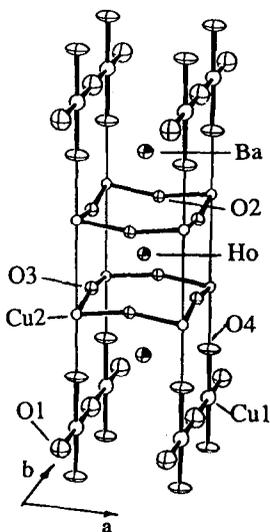
Fig. 2. Structure of  $HoBa_2Cu_3O_{6.8}$  as determined from neutron diffraction data.
