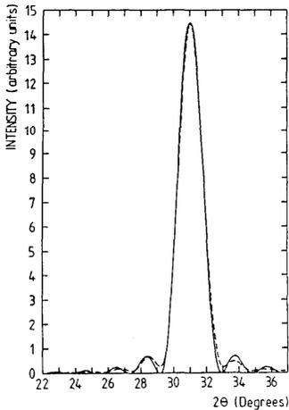
Fig. 2. Experimentally measured x-ray spectrum (dashed line) for a Pb (49 Å) / Ge (59 Å) multilayer fitted with eq. (5) of ref. 14 with  $c^{-1} = 0.04 \text{ \AA}$  (solid line).
