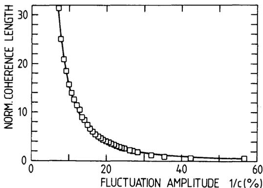
Fig. 4. The number of coherent scattering modulation wavelengths  $\eta$  as a function of fluctuation amplitude using eq. (3) for Nb/Cu multilayers.
