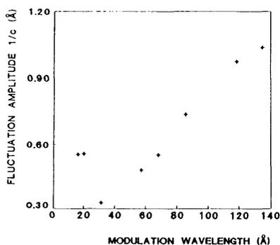
Fig. 5. Fluctuation amplitude  $c^{-1}$  versus modulation wavelength for Nb/Cu multilayers.
