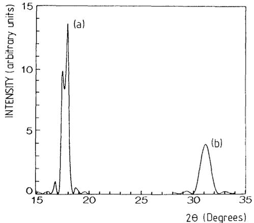
Fig. 3. Simulation of high angle spectra with eq. (5) of ref. 14 for (a)  $d = 5 \text{ \AA}$ ,  $c^{-1} = 0.07 \text{ \AA}$ ,  $N = 25$ ,  $\bar{a} = 28 \text{ \AA}$ ,  $M = 13$ , and (b)  $d = 2.87 \text{ \AA}$  (Pb),  $c^{-1} = 0.07 \text{ \AA}$ ,  $N = 25$ ,  $\bar{a} = 28 \text{ \AA}$ ,  $M = 13$ .
