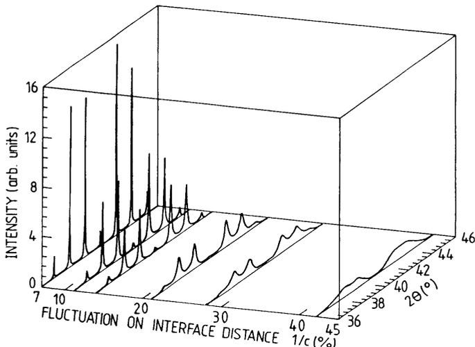
Fig. 1. Evolution of simulated high angle spectra for different values of the fluctuation amplitude  $c^{-1}$ , for  $d_a = 2.33 \text{ \AA}$ ,  $d_b = 2.08 \text{ \AA}$ ,  $N_a = N_b = 24$ ,  $\bar{a} = (d_a + d_b)/2$ .
