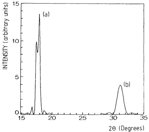
Fig. 3. Simulation of high angle spectra with eq. (5) of ref. 14 for (a)  $d = 5 \text{ \AA}$ ,  $c^{-1} = 0.07 \text{ \AA}$ ,  $N = 25$ ,  $\bar{a} = 28 \text{ \AA}$ ,  $M = 13$ , and (b)  $d = 2.87 \text{ \AA}$  (Pb),  $c^{-1} = 0.07 \text{ \AA}$ ,  $N = 25$ ,  $\bar{a} = 28 \text{ \AA}$ ,  $M = 13$ .
