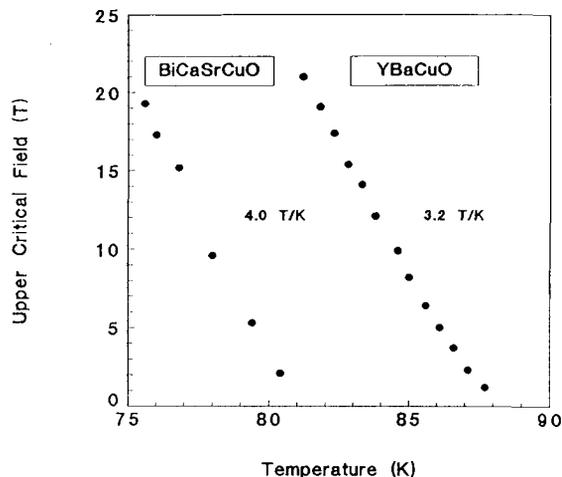
Fig. 2 Temperature dependence of the upper critical field for the BiCaSrCuO sample shown in Fig. 1 and for a typical YBa<sub>2</sub>Cu<sub>3</sub>O<sub>7</sub> sample
