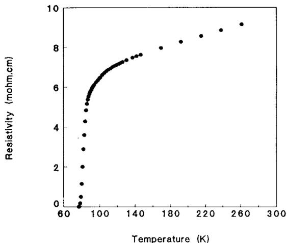
Fig. 1 Temperature dependence of the resistivity for a typical BiCaSrCuO sample
