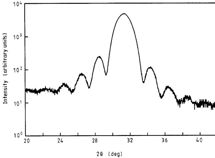
**Figure 2.** The high angle x-ray diffraction profile of a [Pb (45.4 Å)/Ge (29.5 Å)]<sub>5</sub> multilayer. The subscript indicates the number of bilayers. The intensity profile is taken with a  $\frac{1}{8}^\circ$  divergence slit and a 0.15 receiving slit.
