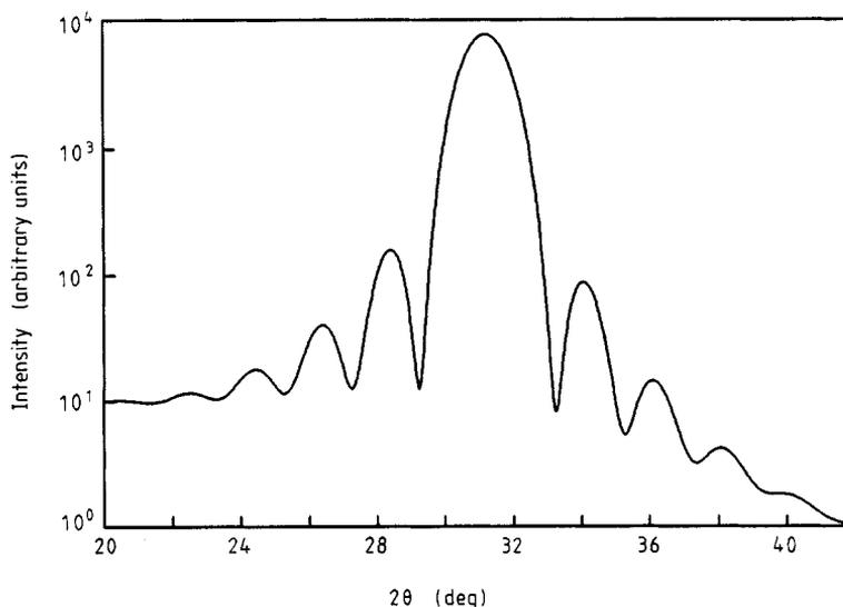
**Figure 4.** The simulation of x-ray high angle diffraction profile for a  $[\text{Pb } (45.4 \text{ \AA})/\text{Ge } (29.5 \text{ \AA})]_5$  multilayer, with  $c_c^- = 3 \text{ \AA}$  and  $c_a^- = 5.5 \text{ \AA}$ , as calculated from equation (6), corrected with Debye-Waller and Lorentz polarisation factors.
