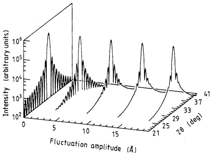
**Figure 3.** The evolution of the x-ray diffraction profile of a Pb (100 Å)/Ge (60 Å) multilayer as a function of  $c_d^{-1}$  using equation (6) when  $c_c^{-1} = 2.5$  Å,  $M = 15$  and  $d = 2.87$  Å.
