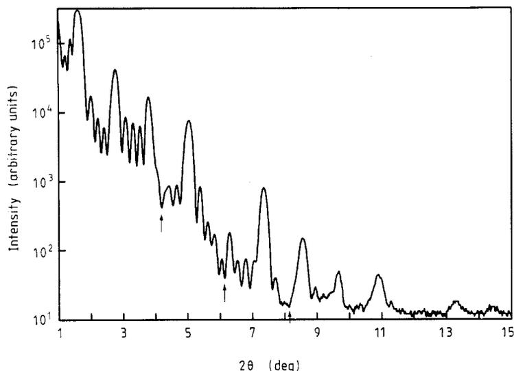
**Figure 1.** The small angle x-ray diffraction profile of a  $[\text{Pb}(45.4 \text{ \AA})/\text{Ge}(29.5 \text{ \AA})]_5$  multilayer. The subscript indicates the number of bilayers. The intensity profile is taken with a  $\frac{1}{4}^\circ$  divergence slit and a 0.15 receiving slit.
