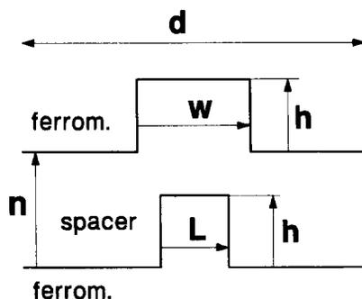
Fig. 1. Illustration of the spatial parameters that characterize the system:  $n$ ,  $h$ ,  $L$ ,  $w$  and  $d$ .
