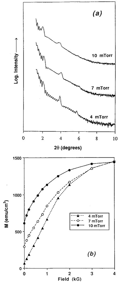
FIG. 1. (a) Low-angle x-ray diffraction spectra and (b) in-plane magnetization curves for  $[\text{Fe}(30 \text{ \AA})/\text{Cr}(12 \text{ \AA})]_{10}$  superlattices sputtered at 4, 7, and 10 mTorr Ar pressure. The x-ray spectra are offset for clarity.
