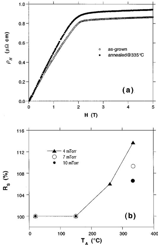
FIG. 4. Room temperature (a) Hall resistivity  $\rho_H$  as a function of field  $H$  for the 7-mTorr sample as-grown and annealed at 335 °C and (b) extraordinary Hall coefficient  $R_s$  as a function of annealing temperature  $T_A$  for the same samples shown in Fig. 1.
