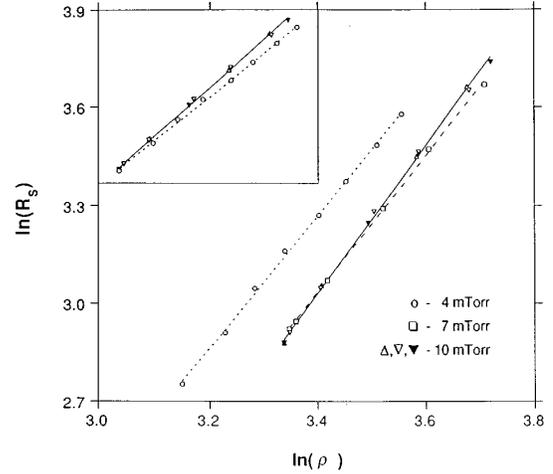
FIG. 3. Log-log plot of the extraordinary Hall coefficient  $R_s$  as a function of longitudinal resistivity  $\rho$  for the same samples shown in Fig. 1. The inset shows the data for the 4-mTorr and 10-mTorr samples offset by a constant.
