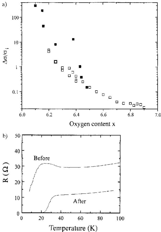
Fig. 2. a) Doping dependence of PPC: Relative change in conductivity  $\Delta\sigma/\sigma_i$  at 95 K as a function of oxygen content  $x$  of  $\text{REBa}_2\text{Cu}_3\text{O}_x$ . Solid symbols refer to  $\text{GdBa}_2\text{Cu}_3\text{O}_x$ , while open symbols refer to  $\text{YBa}_2\text{Cu}_3\text{O}_x$ . b)  $R(T)$  curves before and after illumination for a  $\text{GdBa}_2\text{Cu}_3\text{O}_{6.45}$  sample. The data were obtained from [4].
