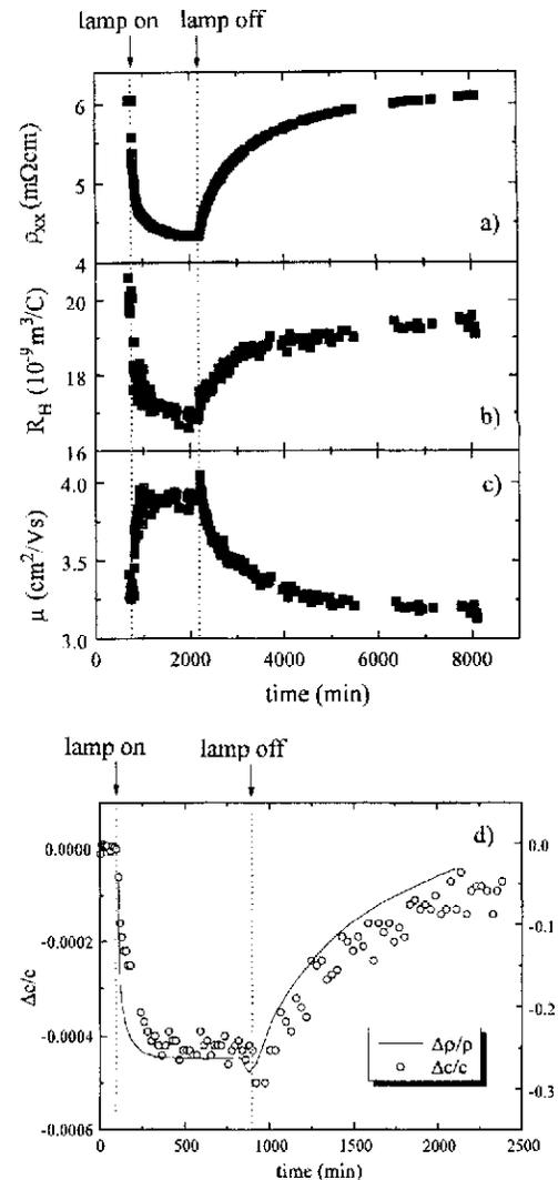
Fig. 3. Time dependence of (a) the resistivity  $\rho_{xx}$ , (b) Hall coefficient  $R_H$ , (c) Hall mobility  $\mu = c(|R_H|/\rho_{xx})$  and (d)  $c$ -axis lattice parameter during excitation and relaxation measured at room temperature in a patterned  $\text{YBa}_2\text{Cu}_3\text{O}_{6.5}$  film. The data were obtained from [5,6].
