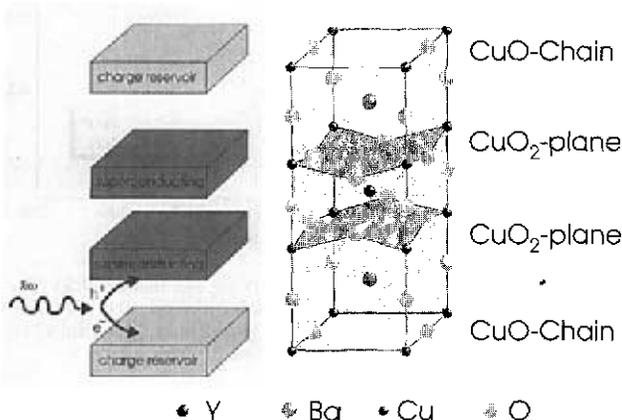
Fig. 1. Structure of  $\text{YBa}_2\text{Cu}_3\text{O}_7$ . The material consists of  $\text{CuO}_2$  planes and  $\text{CuO}$  chains separated by yttrium and barium. The charge carriers responsible for superconductivity are located within the  $\text{CuO}_2$  planes, while the  $\text{CuO}$  chains act as a charge reservoir and their oxygen content determines the carrier concentration in the  $\text{CuO}_2$  planes.
