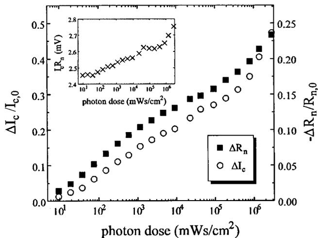
FIG. 4.  $\Delta R_n$  and  $\Delta I_c$  vs photon dose at 5 K.  $R_n$  was measured at 1 mA. The inset shows the change in  $I_c R_n$ .
