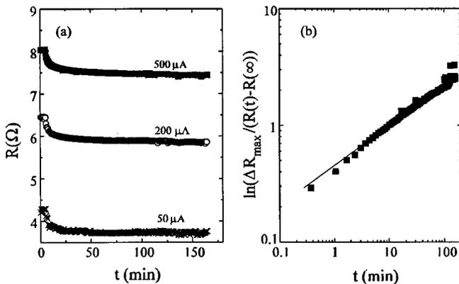
FIG. 2. (a) Time dependence of the dc-SQUID resistance  $R$  during illumination at 70 K.  $R$  was measured at bias currents of 50, 200, and 500  $\mu\text{A}$ . (b) Fit (solid line) of Eq. (1) to the data taken at 500  $\mu\text{A}$ . The fit parameters are  $R(0) = 8.03 \Omega$ ,  $R(\infty) = 7.39 \Omega$ ,  $n_c \tau = 10.2 \text{ min}$ , and  $\beta = 0.34$ .
