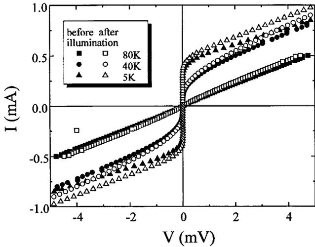
FIG. 1.  $I(V)$  characteristics of the dc-SQUID before and after white light illumination for several different temperatures. Notice the decrease of the normal state resistance  $R_n$  and the increase of the critical current  $I_c$ .
