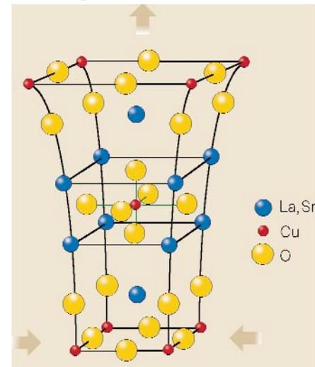
Figure 1  $\text{La}_{1.9}\text{Sr}_{0.1}\text{CuO}_4$  on a substrate that forces it to distort its usual crystal structure (the actual strain is exaggerated here). This distortion can increase the substance's superconducting transition temperature by a factor of two.
