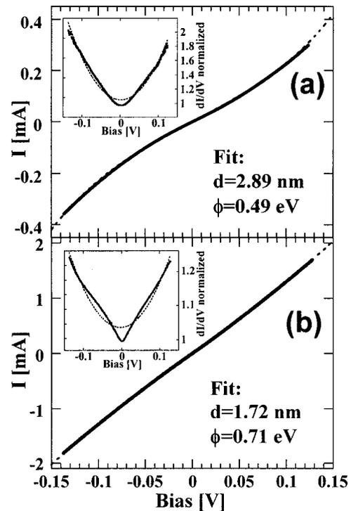
FIG. 1. (a)  $I$ – $V$  curve for sample A at  $T = 90$  K together with a fit to Simmons's model (dashed line). Inset: original conductance data fitted with the BDR model (dashed line). (b) Same for sample B at  $T = 77$  K.
