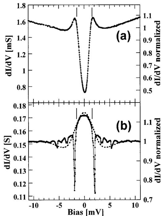
FIG. 2.  $G$ – $V$  data for sample A (a) and B (b) taken at  $T = 4.2$  K. The lines indicate the gap voltage for bulk Nb,  $\pm 1.5$  mV. The dashed line in (b) is data from Ref. 17 for an Fe–Ta point contact with the bias scale multiplied by the gap ratio of Nb to Ta.
