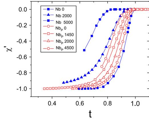
Fig. 2.  $\chi_{ac}(T)$  for the continuous Nb film, Nb (full symbols), and for the porous Nb film,  $Nb_p$  (open symbols), as a function of reduced temperature  $t = T/T_{C0}$ , for different values of applied  $H$ .
