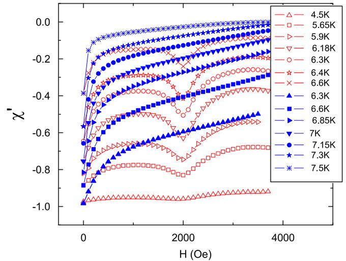
Fig. 3.  $\chi_{ac}(H)$  (ZFC) for both samples at different temperatures, Nb (full) and  $Nb_p$  (open symbols).  $Nb_p$  sample shows matching effects for  $H_1 = 2000 \text{ Oe}$ .
