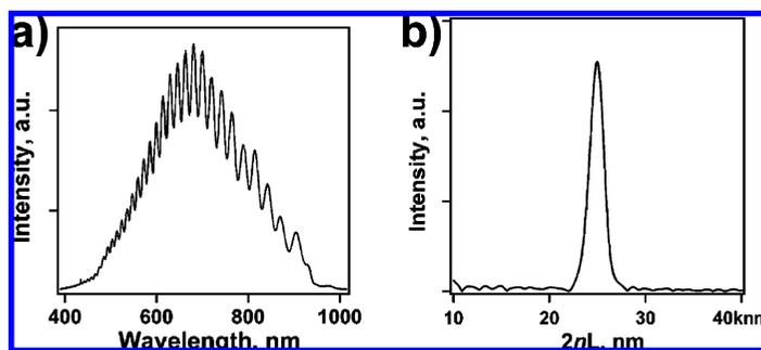
Figure 2. Optical characteristics of a porous alumina thin film. (a) White light reflectance spectrum from a thin film of pAl<sub>2</sub>O<sub>3</sub>. (b) Fourier transform of the reflectance spectrum in (a) results in a single peak whose position along the x-axis corresponds to the effective optical thickness of the thin film,  $2nL$ .
