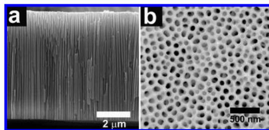
Figure 1. Scanning electron micrographs representative of the porous alumina films used in this study. (a) Cross-sectional view. (b) Plan-view image, showing the entrance to the pores. Average pore diameter is 60 nm, average depth is 6000 nm.
