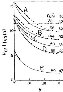
Fig. 2  $H_{C2}(\theta)$  fitted with the de Gennes - MEF expression Eq. (13). Model 1 uses the full expression for  $a'$  (Eq. 11), while Model 2 uses only the normal component of  $a'$  in Eqs. (14) and (15); + is the experimental data.
