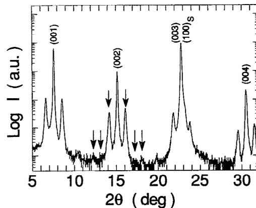
FIG. 6. X-ray diffraction spectra for a  $\text{GdBa}_2\text{Cu}_3\text{O}_{7-\delta}$  (4 unit cells)/ $\text{YBa}_2\text{Cu}_3\text{O}_{7-\delta}$  (4 unit cells)  $\times 21$  superlattice grown on (100) $\text{SrTiO}_3$ . The arrows show the first to third order superlattice satellite peak positions around the (002) reflection. The full width at half-maximum of the rocking curve of the (007) reflection is  $0.23^\circ$ .
