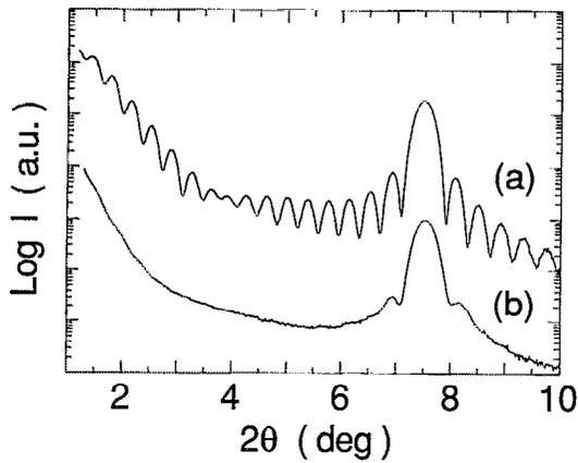
FIG. 2. Low-angle x-ray diffraction spectra of (a) 232 Å  $\text{GdBa}_2\text{Cu}_3\text{O}_{7-\delta}$  thin film grown on (100) $\text{SrTiO}_3$  by the NACHOS method and (b) thin film grown at the same deposition time and conditions as film (a) by the  $0^\circ$  off-axis method.
