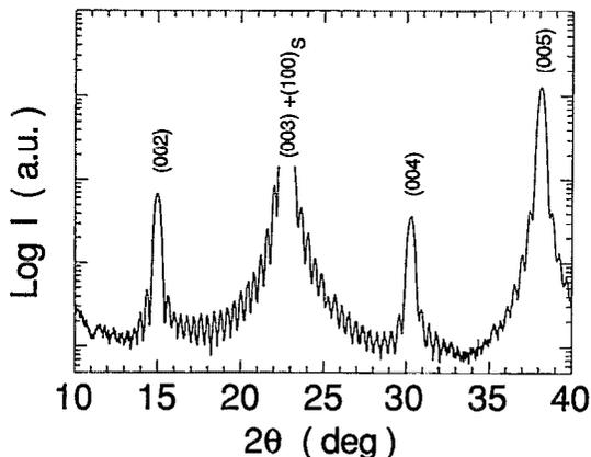
FIG. 3. High-angle x-ray diffraction spectra and the same film shown in Fig. 2(a). Indexing is for  $\text{GdBa}_2\text{Cu}_3\text{O}_{7-\delta}$  peaks;  $(100)_s$  labels the  $(100)\text{SrTiO}_3$  diffraction peak.
