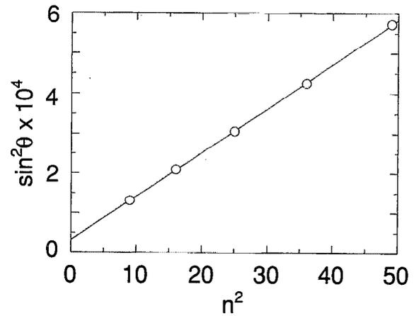
FIG. 4.  $\sin^2\theta$ -vs- $n^2$  plot for the minima below  $3^\circ$  in Fig. 2(a). Solid line is the least-squares linear fit to the data. The film thickness is calculated from this slope (see text for details).
