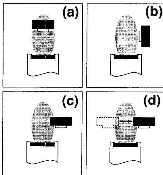
FIG. 1. Schematics of the (a) on axis, (b)  $90^\circ$  off-axis, (c)  $0^\circ$  off-axis, and (d) NACHOS deposition geometries showing the relative positions of target, substrate, and glow-discharge area.
