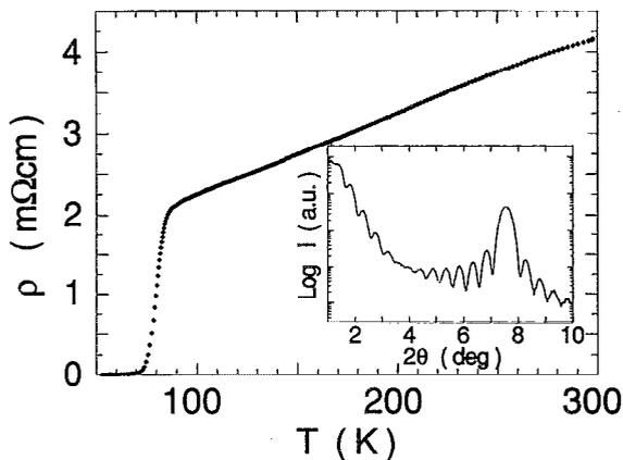
FIG. 5. Resistivity-vs-temperature curve for a 181-Å-thick NACHOS  $\text{GdBa}_2\text{Cu}_3\text{O}_{7-\delta}$  film on (100) $\text{SrTiO}_3$ . Inset shows the low-angle x-ray diffraction spectra of this film.
