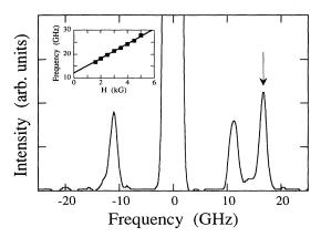
FIG. 2. Brillouin light scattering spectrum for the same  $\Lambda=20$  Å Fe/Cu multilayer shown in Fig. 1 measured in an applied field of 1.6 kG. The arrow indicates the highest-frequency mode. The inset shows the frequency of the high mode versus applied field. The line is a linear least-squares fit to the data based upon a model described in the text. The slope of the line is 3.05 GHz/kG and the intercept 12.1 GHz.
