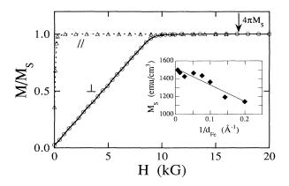
FIG. 1. A room-temperature magnetic hysteresis loop for a  $\Lambda = 20$  Å Fe/Cu multilayer measured parallel and perpendicular to the film. The inset shows the saturation magnetization for equal-layer-thickness Fe/Cu multilayers plotted as a function of the inverse Fe layer thickness. The line is a linear least-squares fit to the data based upon a model described in the text.
