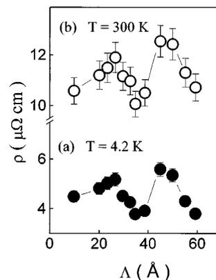
FIG. 1. Average resistivity for a series of  $(\text{Co}_{0.6\Lambda}/\text{Ni}_{0.4\Lambda})_N$  as a function of  $\Lambda$  in Å at two different temperatures, (a)  $T=4.2$  K and (b)  $T=300$  K. The solid lines are guides to the eye.
