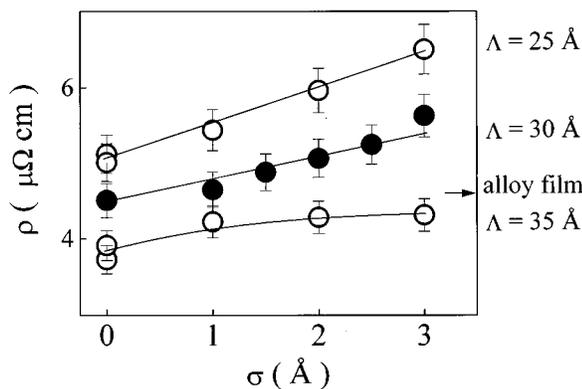
FIG. 3. Average resistivity for  $(\text{Co}_{0.6\Lambda}/\text{Ni}_{0.4\Lambda})_N$ ,  $\Lambda=25, 30,$  and  $35 \text{ \AA}$  as a function of layer thickness variation,  $\sigma$ . The arrow indicates Co/Ni alloy resistivity. The solid lines are guides to the eye.
