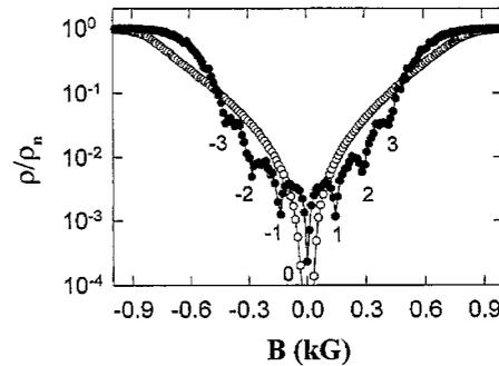
Fig. 3. Field dependence of the resistivity of a 100 nm thick Nb film with a Ni dot array of spacing  $d = 410$  nm (filled symbols) and in a reference only Nb area (hollow symbols), both measured with  $J = 2.5 \times 10^4$  A/cm<sup>2</sup> at 8.2 K. The resistivity has been normalized by the normal state resistivity  $\rho_n$ . The order  $n$  of the matching fields  $B_n$  are indicated.
