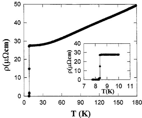
Fig. 2. Temperature dependence of the resistivity of a 100 nm thick Nb film with an array of Ni dots ( $d = 410$  nm). Inset shows the details of the superconducting transition.
