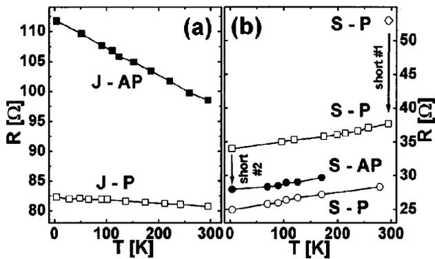
FIG. 1. (a)  $R(T)$  for sample J in both the antiparallel (■) and parallel (□) magnetic states; (b) same for sample S. Open diamond and arrow show  $R$  before and after the first short was introduced. Small contact,  $P$  state (□); large contact, AP state (●); large contact,  $P$  state (○).
