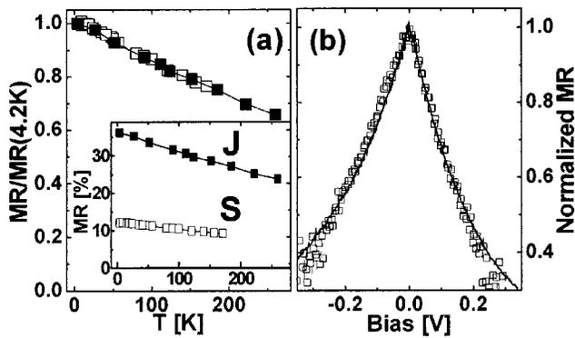
FIG. 4. (a)  $T$  dependence of the normalized differential MR for sample J (■) and S (□). Inset: same data before normalization; (b) bias dependence of the differential magnetoresistance of sample J (—), and S (□).
