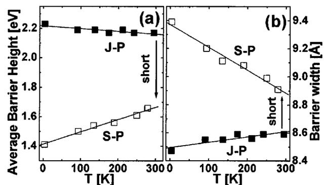
FIG. 3. Average barrier height (a) and barrier width (b) vs  $T$  for sample J (■) and S (□) in the parallel state. Straight lines are guides to the eye.
