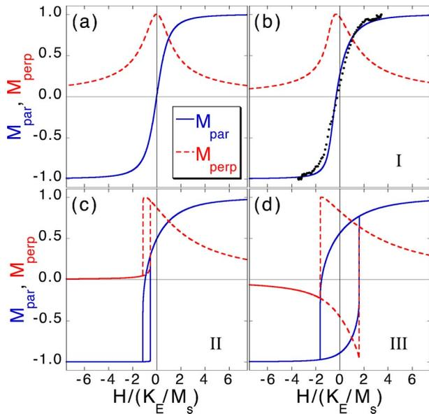
FIG. 2. (Color online) Hysteresis loops from the coherent rotation model with  $\theta_E$  and  $\theta_u$  fixed to  $90^\circ$  and  $45^\circ$ , respectively. Shown are the longitudinal (solid line) and transverse (dashed line) magnetizations  $M_{par}$  and  $M_{perp}$  normalized by the saturation magnetization. The curves are for  $K_u/K_E$  ratios of 0 (a), 0.3 (b), 0.95 (c), and 1.5 (d). The solid symbols in (b) indicate the average of the two hysteresis branches from Fig. 1(d).
