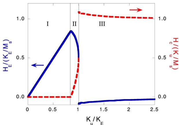
FIG. 3. (Color online) Calculated  $H_E$  (solid line) and  $H_c$  (dashed line) normalized by  $K_E/M_s$  and  $K_u/M_s$ , respectively, as a function of  $K_u/K_E$  at fixed  $\theta_E=90^\circ$  and  $\theta_u=45^\circ$ . The regions of different hysteresis behavior are indicated by I, II, and III.
