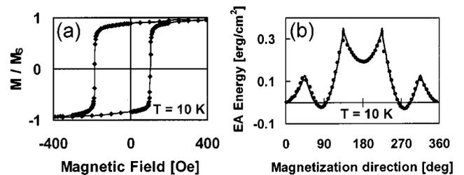
FIG. 1. (a) Hysteresis loop of Fe/MnF<sub>2</sub> bilayer at  $T = 10 \text{ K}$ ; the line is a guide to the eye. (b) Angular dependence of the exchange anisotropy energy per area of Fe/MnF<sub>2</sub> bilayer at  $T = 10 \text{ K}$ . Circles are experimental data obtained by the AMR technique; the line is a fit to the experimental data using Eq. (2) and a phenomenological uniaxial anisotropy term  $K_2 \cos(2\alpha_F)$ .
