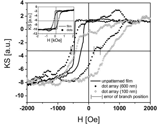
FIG. 2. MOKE signal (KS) of  $M_l$  vs  $H$  of unpatterned Fe-FeF<sub>2</sub> film and different Fe dot arrays on FeF<sub>2</sub> at 10 K (below  $T_N$ ). The inset shows the signal of unpatterned Fe-FeF<sub>2</sub> film and the 600 nm Fe dots on FeF<sub>2</sub> at 90 K (above  $T_N$ ).
