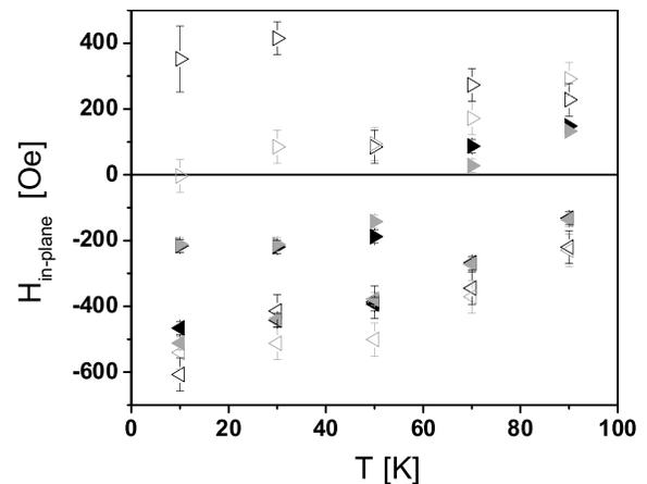
FIG. 3. In-plane magnetic field component  $H_{\text{in-plane}}$  for the positions of the DB (triangles pointing to the left) and IB (triangles pointing to the right), defined by  $H(M_l = 0)$ , for unpatterned (solid symbols) and patterned (open symbols) sample. For the black symbols the field was parallel to the sample surface. For the gray symbols the field was tilted by  $40^\circ$  with respect to the surface after field cooling.
