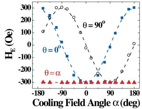
FIG. 7. (Color online) Exchange field  $H_E$  at 15 K vs cooling field angle  $\alpha$  for Ni/polycrystalline- $\text{FeF}_2$ , for measurements along  $\theta=0^\circ$  (blue squares),  $90^\circ$  (black circles), and  $\alpha$  (red triangles). Dashed lines are guides to the eye.
