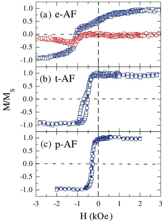
FIG. 2. (Color online) Longitudinal (blue squares) and transverse (red circles) magnetic hysteresis loops measured at 15 K along  $\theta=0^\circ$  of (a) Ni/epitaxial- $\text{FeF}_2$  when  $\alpha=30^\circ$ , (b) Ni/twinned- $\text{FeF}_2$  when  $\alpha=35^\circ$  (longitudinal only), (c) polycrystalline  $\text{FeF}_2/\text{Fe}$  when  $\alpha=20^\circ$  (longitudinal only).
