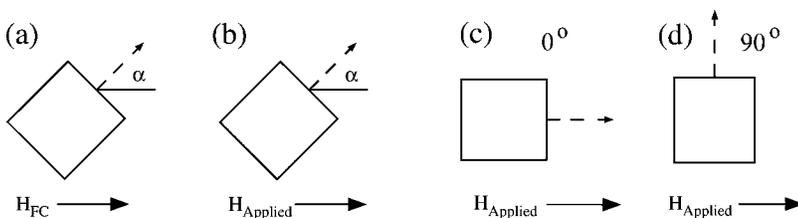
FIG. 1. Sample geometries relative to the 0° line (dashed arrow, defined in Table I) during (a) field cooling along angle  $\alpha$  and measurement along  $\theta =$  (b)  $\alpha$ , (c) 0°, and (d) 90°.
