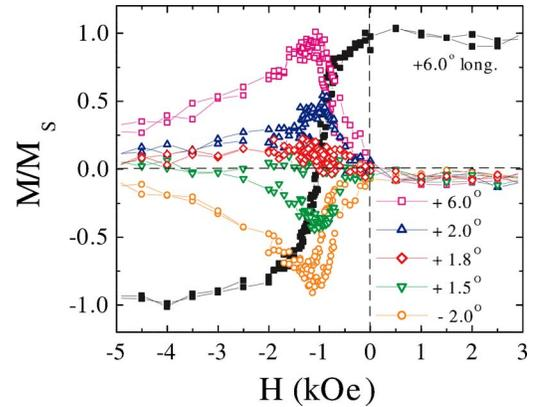
FIG. 5. (Color online) Hysteresis loops measured at different  $\theta$  angles when  $\alpha=0^\circ$  and  $H_{\text{FC}}=1$  kOe. The transverse loop is flat at  $\theta=1.8^\circ$ . The transverse loop peaks grow as  $\theta$  changes from  $1.8^\circ$  to  $6.0^\circ$ . A longitudinal loop measured at  $\theta=6.0^\circ$  (black squares) is shown for comparison.
