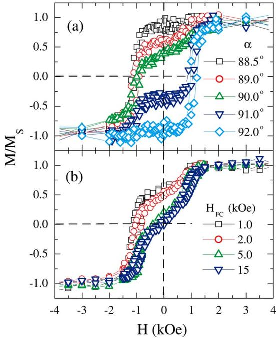
FIG. 4. (Color online) (a) Longitudinal hysteresis loops measured at  $\theta=0^\circ$  when the field cooling angle is  $88.5^\circ \leq \alpha \leq 92.0^\circ$ . The magnetization associated with each subloop changes as  $\alpha$  varies around  $90^\circ$ . (b) Longitudinal hysteresis loops measured at  $\theta=0^\circ$  when the field cooling angle is  $\alpha=89^\circ$ . As  $\alpha$  is increased, the positively biased loop grows at the expense of the negatively biased loop.
