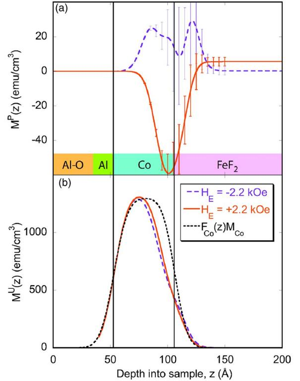
FIG. 7. (Color online) (a) *Pinned* and (b) *unpinned* magnetization depth profiles are shown for the cases of  $H_E = -2.2$  kOe (dashed curve) and  $H_E = +2.2$  kOe (solid curve). The short-dashed curve represents the product of the depth profile of the fraction of Co atoms  $F_{\text{Co}}$  and  $M_{\text{Co}}$ . The vertical lines are located at the centers of the Al/Co and Co/ $\text{FeF}_2$  chemical interfaces.
