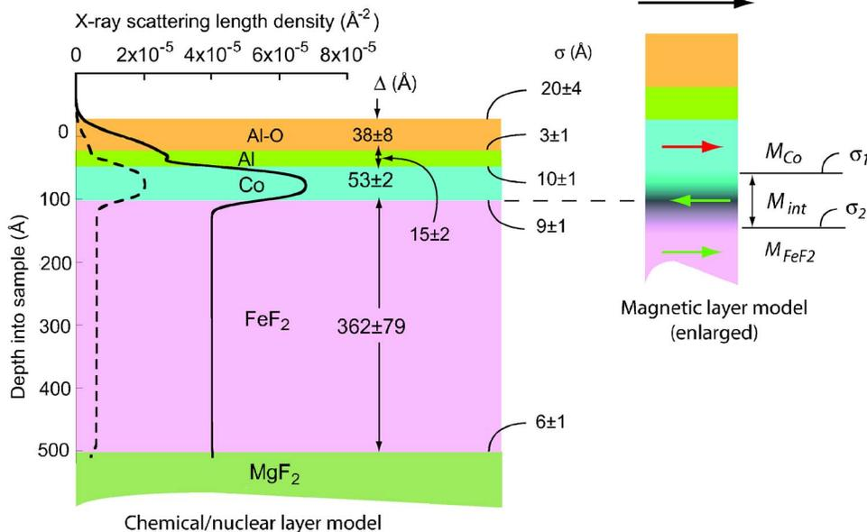
FIG. 2. (Color online) Left: The chemical/nuclear model structure showing the chemical layers, their thickness ( $\Delta$ ) and interface roughness ( $\sigma$ ). The real (solid curve) and imaginary (dashed) components of the x-ray scattering length density are shown. Right: The scattering model is shown.
