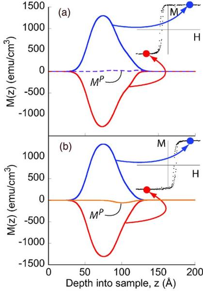
FIG. 6. (Color online) Net magnetization depth profiles for  $H_A = +7$  kOe (blue curve) and  $H_A = -7$  kOe (red curve) and (a)  $H_E = -2.2$  kOe and (b)  $H_E = +2.2$  kOe. The *pinned* components of the magnetization depth profiles are shown as the dashed purple and orange curves and in greater detail in Fig. 7(a).
