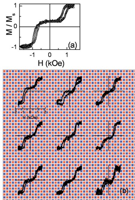
FIG. 2. (Color online) Protocol II. (a) MOKE loop at  $T=20$  K illuminating the whole sample after cooling from room temperature at intermediate  $H_{FC}=1$  kOe. (b) Spatially resolved MOKE loops at different positions. Illustrated color-coded background as in Fig. 1.
