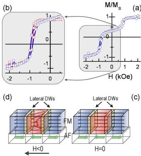
FIG. 3. (Color online) (a) DHL for intermediate  $H_{FC}=1$  kOe. (b) Comparison between a *single loop* (low  $H_{FC}=0.5$  kOe) (squares) and the rescaled *negative-biased subloop* from (a) (circles). Both loops were measured by SQUID at 10 K. (c) Illustrated spin configuration at  $H=0$  and (d)  $H<0$ . Blue (left and right) and red (middle) domains yield positive and negative EB, respectively.
