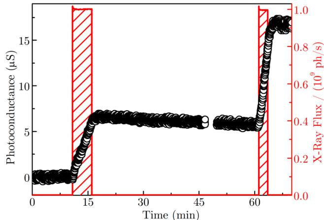
FIG. 1. (Color online) Photoconductance (black circles) of the  $\text{VO}_2$  device at 300 K, showing rapid increase during x-ray illumination (dashed red region) as well as slow decrease after the x-ray illumination was turned off.
