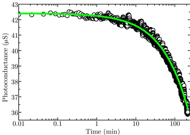
FIG. 3. (Color online) Decay of photoconductance at 330 K postillumination. The green line is a fit using a stretched exponential with the additional information that the photoconductance eventually returns to zero. The mean relaxation time is 69 hours.
