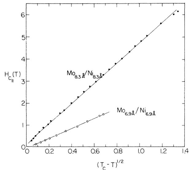
FIG. 3. Parallel critical field exhibiting a  $(T_c - T)^{1/2}$  temperature dependence.
