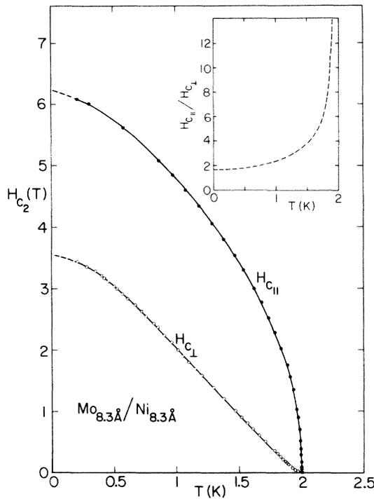
FIG. 1. Temperature dependence of the parallel  $H_{c||}$  and perpendicular  $H_{c\perp}$  critical fields for Mo-Ni heterostructures with  $\lambda = 16.6 \text{ \AA}$ . Inset shows critical field anisotropy. X-ray structural data indicate that layering is preserved in this structure.
