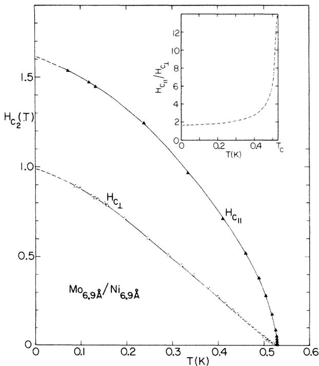
FIG. 2. Temperature dependence of the parallel  $H_{c||}$  and perpendicular  $H_{c\perp}$  critical fields for structure with  $\lambda = 13.8 \text{ \AA}$ . Inset shows critical field anisotropy. X-ray structural data reveal a typical glassylike diffraction pattern, signaling a structural collapse.
