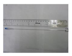
2.- Insert your sample inside the tube. **Typically 50 to 100** mg (maximum).
