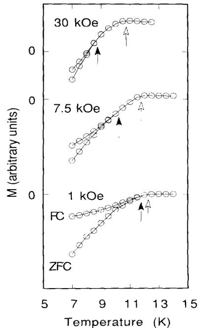
Fig. 1. ZFC and FC magnetization for sample 2 as a function of temperature. Data for  $H=1$  kOe, 7.5 kOe and 30 kOe are included. Open arrows indicate the onset of the diamagnetic signal, i.e. the upper critical field. Full arrows indicate the temperature at which irreversibility begins, i.e. the irreversibility point.
