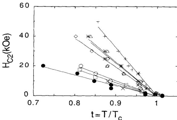
Fig. 2. Critical field,  $H_{c2}$ , as a function of reduced temperature,  $t$ . Solid lines indicate linear fits to the data. (○) sample 1a, (□) sample 1b, (×) sample 1c, (★) sample 2, (+) sample 3, (△) sample 4, (×) sample 5a and (◇) sample 5b.
