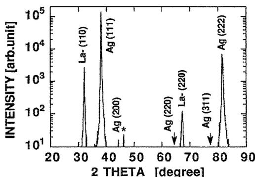
FIG. 4. XRD spectra of  $\text{Ag}/\text{LaBa}_2\text{Cu}_3\text{O}_y/\text{Ag}$  trilayer on sapphire (1120). The reflection peak with an asterisk is  $\text{LaBa}_2\text{Cu}_3\text{O}_y$  (200), (020), or (006) peak. A small Ag (200) peak is also observed; the expected peak positions for the Ag (220) and (311) are also shown with arrows.
