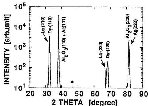
FIG. 3. XRD spectra of  $\text{DyBa}_2\text{Cu}_3\text{O}_y/\text{LaBa}_2\text{Cu}_3\text{O}_y/\text{Ag}$  trilayer on sapphire (1120) substrate. The small reflection peak with an asterisk is (200), (020), or (006) peak of  $\text{LaBa}_2\text{Cu}_3\text{O}_y$  or  $\text{DyBa}_2\text{Cu}_3\text{O}_y$  films.
