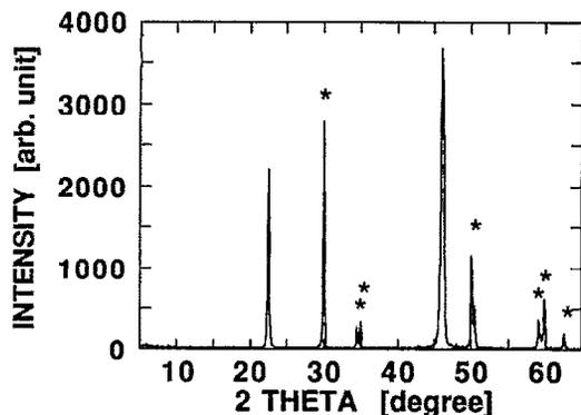
FIG. 1. XRD spectra of  $\text{LaBa}_2\text{Cu}_3\text{O}_y$  film grown on a polycrystalline YSZ substrate at  $450^\circ\text{C}$ . Asterisks show the reflection peaks of YSZ substrate.
