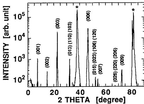
FIG. 5. XRD spectra of  $\text{LaBa}_2\text{Cu}_3\text{O}_y/\text{Ag}$  bilayer on sapphire  $(11\bar{2}0)$  with  $\text{LaBa}_2\text{Cu}_3\text{O}_y$  layer deposited at a substrate temperature of  $560^\circ\text{C}$ . Asterisks show the peaks of Ag layer and sapphire substrate.
