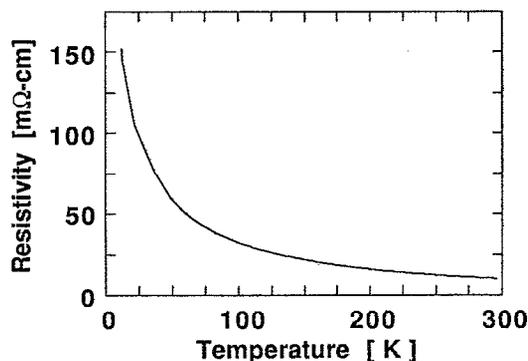
FIG. 2. Resistivity vs temperature curve of  $\text{LaBa}_2\text{Cu}_3\text{O}_y$  film grown on polycrystalline YSZ substrate at  $450^\circ\text{C}$ .
