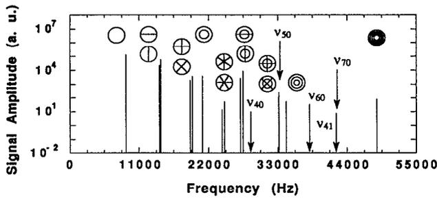
FIG. 2. Signal amplitude vs the square of frequency for a  $\sim 15.5 \mu\text{m}$  aluminum film. The configurational representation of each mode is shown above its resonant peak. The arrows point at missing modes. These modes are labeled with  $\nu_{ij}$ 's;  $i$  and  $j$  are, respectively, the number of nodal circles and lines.
