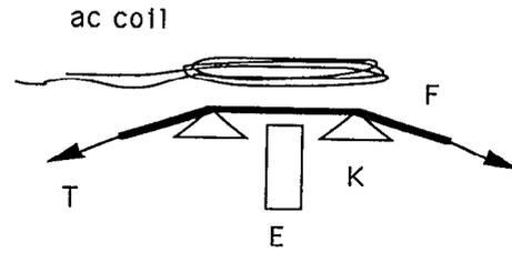
FIG. 1. Schematic diagram of the vibrating membrane device.  $F$  is the film,  $T$  is tension,  $K$  is the circular knife-edge support, and  $E$  is the receiver electrode.
