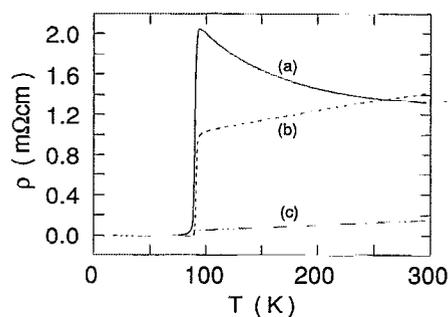
FIG. 3. Resistivity vs temperature curves of  $\text{GdBa}_2\text{Cu}_3\text{O}_{7-\delta}$  films with (a)  $a$ - oriented by the two-step- $T_s$  method, (b)  $b$ -axis oriented by the two-step- $T_s$  method, and (c) typical  $c$ -axis oriented film.
