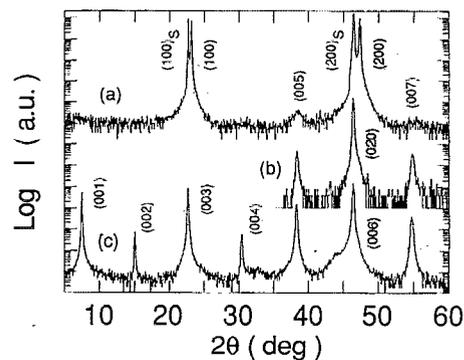
FIG. 2. Representative  $\theta$ - $2\theta$  XRD spectra for  $a$ -,  $b$ -, and  $c$ -axis  $\text{GdBa}_2\text{Cu}_3\text{O}_{7-\delta}$  films on (100)  $\text{SrTiO}_3$ ,  $b$ -axis film was grown on 18° faceted (100)  $\text{SrTiO}_3$  and XRD spectra were taken around the [100]  $\text{SrTiO}_3$  direction. Indexing in the figure for  $\text{GdBa}_2\text{Cu}_3\text{O}_{7-\delta}$  films; (100)<sub>s</sub> and (200)<sub>s</sub> denote  $\text{SrTiO}_3$  reflections.
