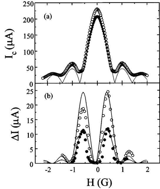
FIG. 3. Magnetic field dependence of the Fiske step (b) before (black dots) and after illumination (white dots) as compared to the Fraunhofer pattern (a). The solid lines in (b) are the theoretical curves  $F_1^2$  (see Eq. 3) and in (a) are  $|\sin \pi\phi/\pi\phi|$ .
