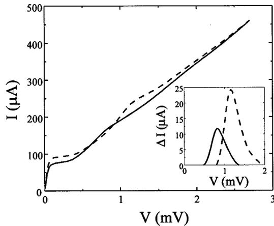
FIG. 2.  $I(V)$  characteristics of a  $\text{YBa}_2\text{Cu}_3\text{O}_x$  GBJJ before (solid line) and after illumination (dotted line) for an applied magnetic field of  $H=0.56$  G at  $T=12$  K. The inset shows the Fiske step before (solid line) and after illumination (dotted line) when the background is subtracted.
