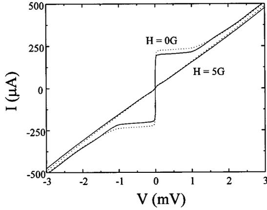
FIG. 1.  $I(V)$  characteristics of a  $\text{YBa}_2\text{Cu}_3\text{O}_x$  GBJJ before (solid line) and after illumination (dotted line) without applied magnetic field at  $T=12$  K. The normal state resistance is shown before (solid line) and after illumination (dotted line) for an applied magnetic field of 5 G.
