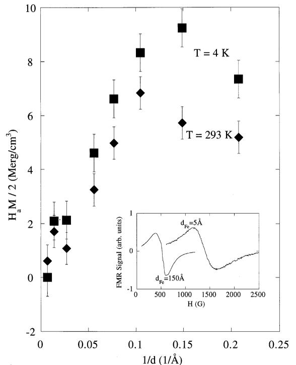
Fig. 3. Intrinsic anisotropy energy as a function of inverse Fe layer thickness. (See model in text.) Error bars are estimates obtained from uncertainties in magnetization and resonance position. Note deviation from linearity for the thinnest samples.
