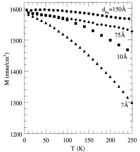
Fig. 1. Magnetization versus temperature for  $d_{\text{Fe}} = 150 \text{ \AA}$  (circles),  $75 \text{ \AA}$  (diamonds),  $10 \text{ \AA}$  (squares) and  $7 \text{ \AA}$  (triangles) samples.
