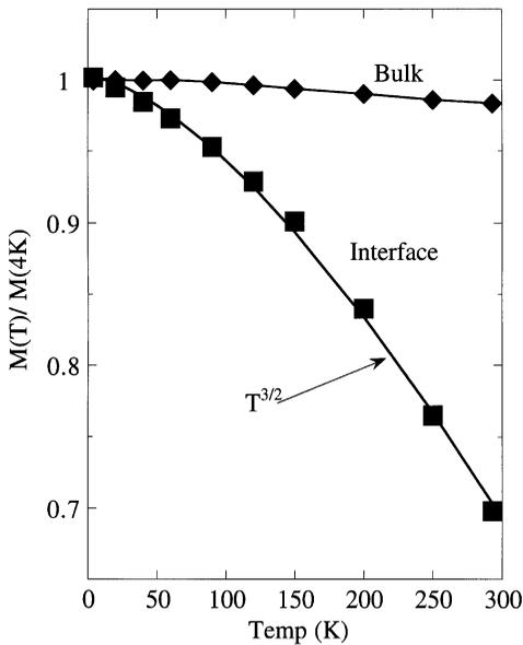
Fig. 2. Reduced interface (squares) and bulk (diamonds) magnetization versus temperature. Error bars are comparable to the size of the markers and are estimated from uncertainties in the SQUID signal. The solid line is a fit to the Bloch Law model.
