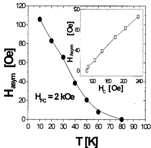
FIG. 4. The temperature dependence of  $H_{\text{asym}}$  (as defined in Fig. 3) for  $H_{\text{FC}}=2$  kOe. Inset:  $H_{\text{asym}}$  vs coercivity,  $H_C$ . The solid lines are guides to the eye.
