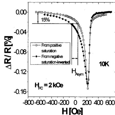
FIG. 3. The inversion and overlaying of the “increasing field” and “decreasing field” parts of the AMR trace shown in Fig. 1(a). The definition of the parameter  $H_{asym}$  is clearly illustrated. The solid lines are guides to the eye.
