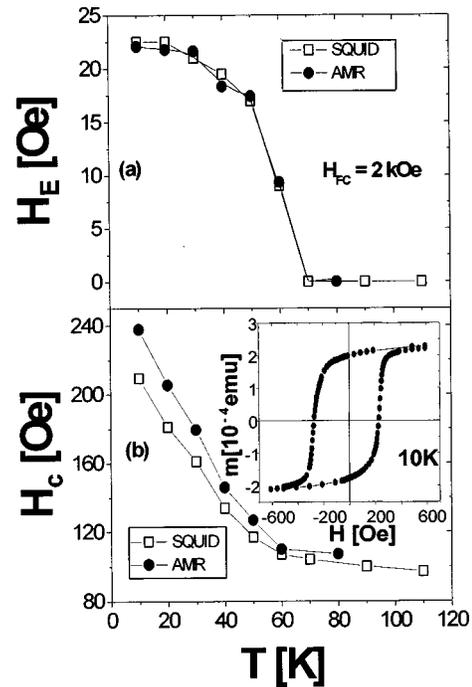
FIG. 2. The temperature dependence of the exchange bias (a) and coercivity (b) for  $H_{FC}=2$  kOe. Square symbols represent data taken via SQUID magnetometry while circular symbols represent data taken via AMR measurements. Inset: SQUID hysteresis loop at  $H_{FC}=2$  kOe and  $T=10$  K. The solid lines are guides to the eye.
