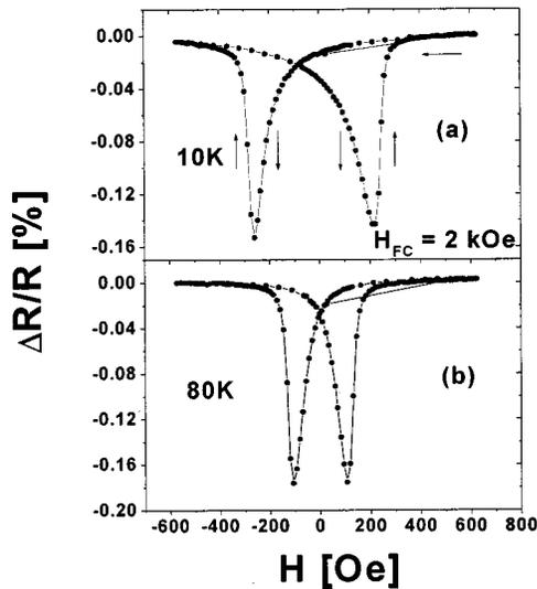
FIG. 1. Fractional MR at (a)  $T=10$  and (b)  $80$  K. The cooling field,  $H_{FC}=2$  kOe. Note that the data were taken with the current in plane and parallel to the in-plane magnetic field. The solid lines are guides to the eye. Arrows show the direction in which the field was swept.
