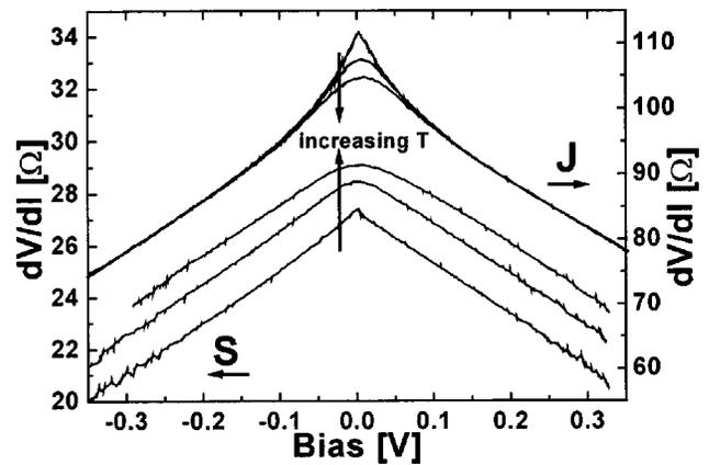
FIG. 2. Differential resistance vs applied bias at 4.2, 90, and 155 K, respectively. Three top curves: sample J; three bottom curves: sample S.
