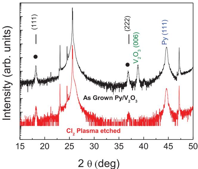
FIG. 7. (Color online) X-ray diffraction patterns for a bilayer Py (30 nm)/ $V_2O_3$  (100 nm) as grown (top black) and after etching (bottom red). Diffraction maxima from  $V_2O_3$  and Py are labeled in the figure; diffraction maxima shown by the black dots are from an unexpected phase. Peak positions from  $Fe_3O_4$  (111) planes are marked at the top. All other diffraction maxima not marked in the figure are due to the r-cut sapphire substrate.
