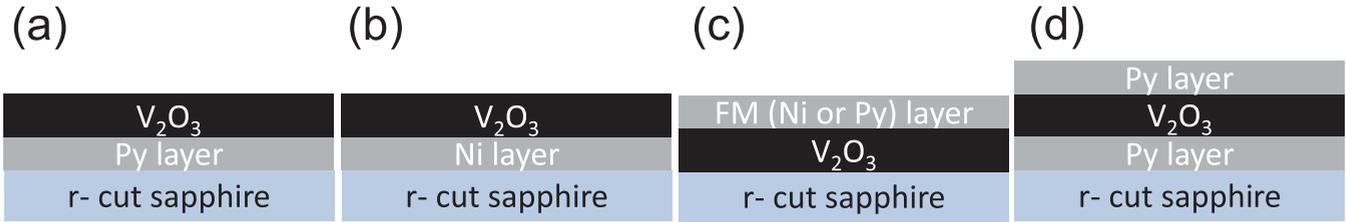
FIG. 1. (Color online) Schematic model of different samples studied. (a) and (b) Py or Ni was deposited at room temperature. The  $V_2O_3$  layer was deposited later at  $750^\circ\text{C}$  after a  $7\text{ K/min}$  heating ramp. (c) The  $V_2O_3$  layer was deposited at  $750^\circ\text{C}$  and the top FM at room temperature. (d) Trilayer used for MOKE measurements.
