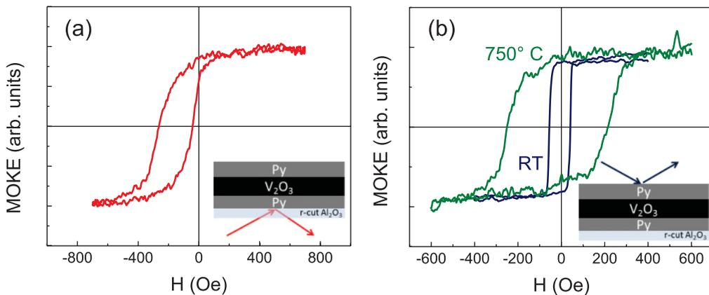
FIG. 9. (Color online) MOKE hysteresis loops at 10 K after cooling the sample, with a field of 1000 Oe. (a) MOKE probing the bottom Py layer. (b) MOKE probing the top Py layer deposited at room temperature and at 750 °C. Insets show MOKE probing each FM individual layer.
