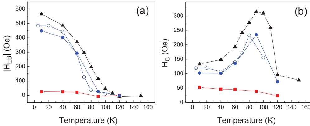
FIG. 6. (Color online) (a) Dependence of the EB field with temperature. (b) Dependence of the coercive field with temperature. Py (30 nm)/ $V_2O_3$  (100 nm) bilayers are measured with SQUID (solid black triangles), Py (30 nm)/ $V_2O_3$  (50 nm) is measured with SQUID (solid blue circles), Py (30 nm)/ $V_2O_3$  (50 nm) is from MR measurements (open blue circles), and Py (30 nm)/ $V_2O_3$  (25 nm) is measured with SQUID (solid red squares).
