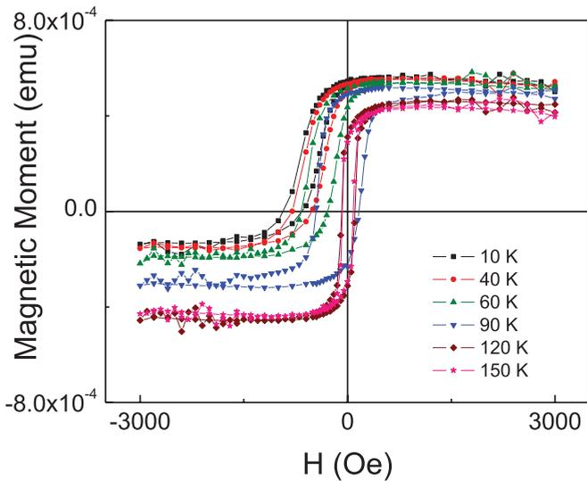
FIG. 3. (Color online) Hysteresis loops at different temperatures in Py (30 nm)/V<sub>2</sub>O<sub>3</sub> (100 nm) bilayers. The sample was cooled from room temperature to 10 K with a field of 1000 Oe.
