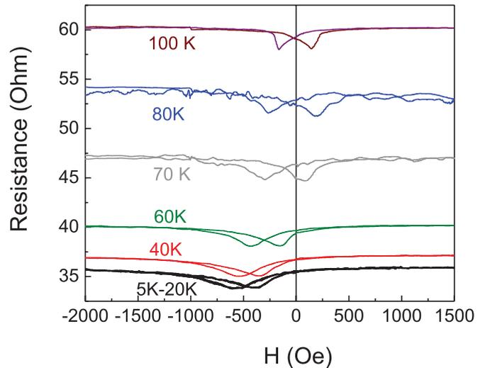
FIG. 5. (Color online) MR measurements at different temperatures in Py (30 nm)/V<sub>2</sub>O<sub>3</sub> (50 nm). The sample was cooled from 300 to 4.2 K with an applied field of 1000 Oe.
