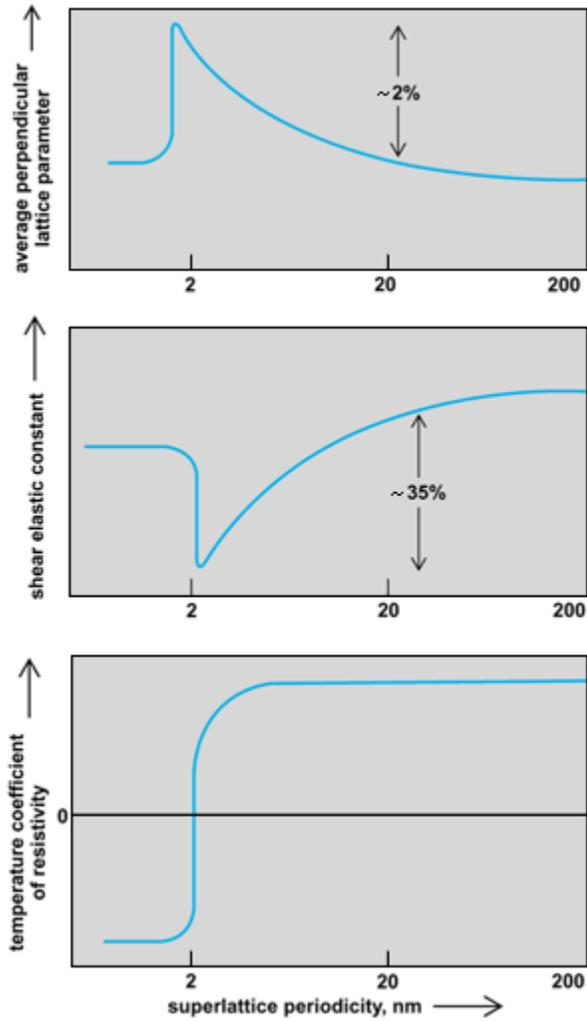
**Fig. 2** Average perpendicular lattice parameter, shear elastic constant, and temperature coefficient of resistivity versus superlattice periodicity. (After M. R. Khan et al., *Structural, elastic and transport anomalies in molybdenum-nickel superlattices*, *Phys. Rev.*, B27:7186–7193, 1983)
