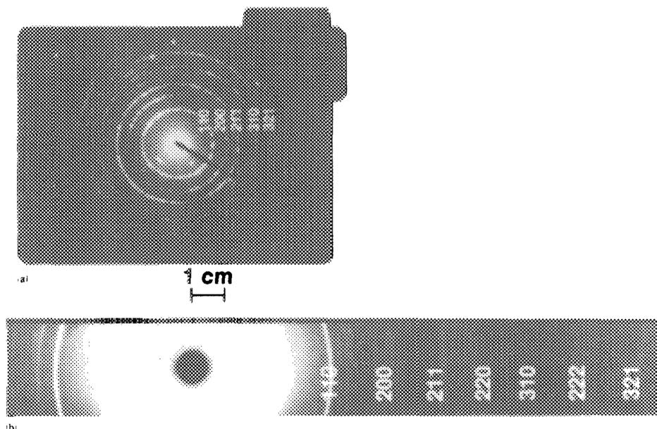
FIG. 4. (a) Electron diffraction picture of a W-C multilayer after crystallization showing seven distinct tungsten rings. (b) Corresponding Debye-Scherrer picture, showing also some weak Si or unidentified additional rings.
