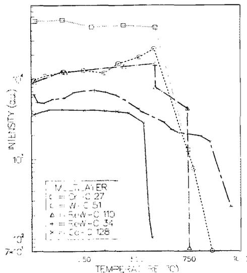
FIG. 3. Intensity of the first order Bragg peak as a function of temperature.
