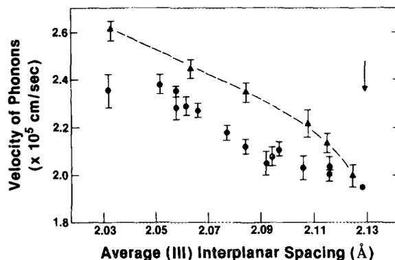
FIG. 1. Velocity of phonons vs average nickel [111] interplanar spacing. Dots are measured values by Brillouin scattering and triangles are values from molecular dynamics calculations. The arrow indicates the value at which the structure becomes highly disordered in the Mo/Ni superlattices and where the molecular dynamics crystal fails.
