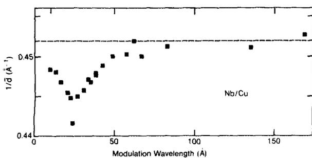
FIG. 2. Reciprocal of the average lattice spacing  $\bar{d}$  vs modulation wavelength for Nb/Cu superlattices.
