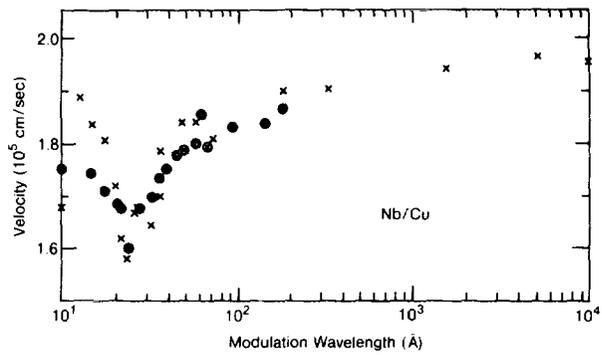
FIG. 3. Surface wave velocity of N/Cu superlattices as a function of modulation wavelength. Crosses are experimental results from Ref. 8 and dots are the values calculated as described in the text.
