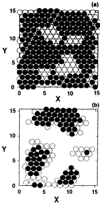
Fig. 2. Arrangements of atoms after the deposition of 680 atoms at  $T_S=0$ . (a) Atoms in the first deposited layer on top of the movable substrate layer. (b) Atoms in the fifth deposited layer on top of the fourth layer.
